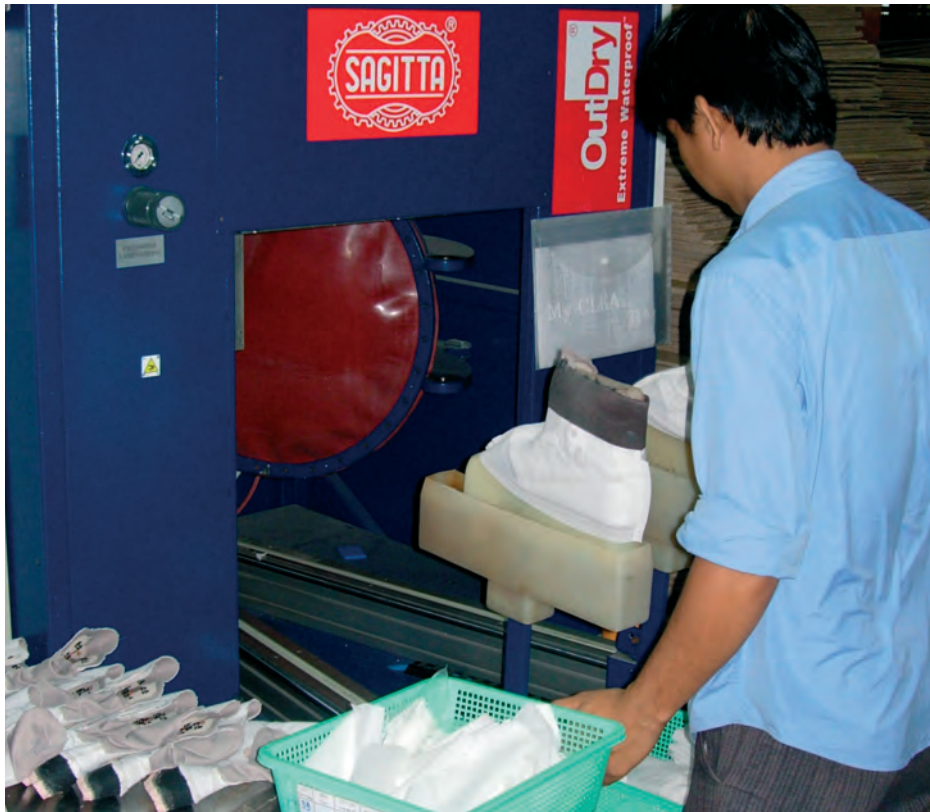
Machine bonding of the OutDry membrane to the inside of the upper
